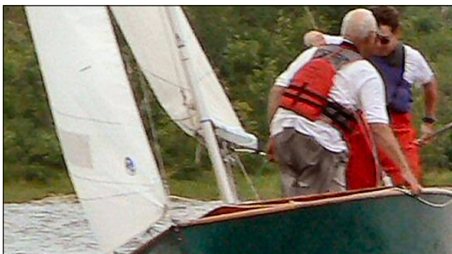
5. (above) Helm turns to face forward. As he completes his 180° turn, his tiller arm briefly ends up behind his back (below). Crew meanwhile, faces aft to initiate his turn. Note how both sails are slightly eased. At this point, neither helm nor crew is watching the sails which are being trimmed by "feel", such as angle of heel, wind strength, etc.
