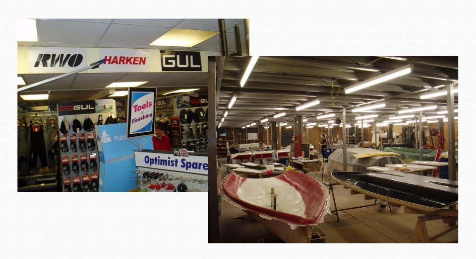
The Master "plug" from which all the official moulds are made (essentially a complete Wayfarer Hull that will never sail). Two moulds are needed from this Master – the hull bottom and the interior.
