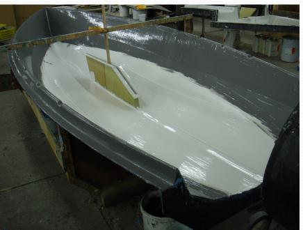
It is at this point that the major difference in construction and cost between cruising/training models and race boats occurs. 10mm, closed cell, rigid foam is installed in race models to increase stiffness (and cost as well).
