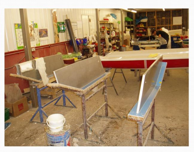
Centre Board trunk and taping for waterline put in freshly cleaned and waxed mould. Pictured is a "Gull" but same process is used for Wayfarer.
